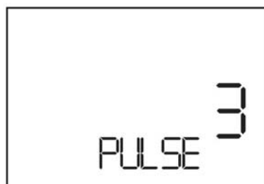
Fig.11 Adjustment of impulses for each complete turn of the wheel
